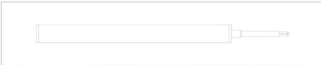
(1) Power cable in rear feed.
