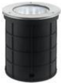
IL8110 E27 socket IP67 Tempering glass diffuser Silicone gasket, plastic housing 304 stainless steel frame D: 150mm H: 270mm
