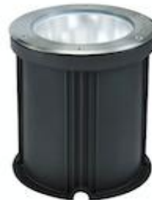
IL8101 E27 socket IP67 Tempering glass diffuser Silicone gasket, plastic housing 304 stainless steel frame D: 260mm H: 330mm
