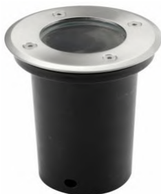
IL8302 GU10 socket IP67 Tempering glass diffuser Silicone gasket, plastic housing 304 stainless steel frame D: 110mm H: 97mm
